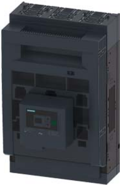
FUSE-SWITCH-DISCONNECTOR 3-POLE, NH1, 250A MOUNTING PLATE CONSTRUCTION COVER LEVEL 70 MM BOX TERMINAL FUSE MONITORING ELECTRONIC, EFM 20
