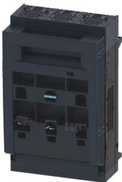
FUSE-SWITCH-DISCONNECTOR 3-POLE, NH1, 250A 60MM BUSBAR SYSTEM COVERS FOR RITTAL FLAT CONNECTOR
