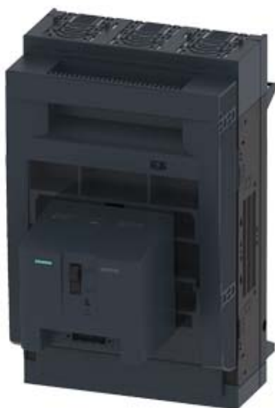
FUSE-SWITCH-DISCONNECTOR 3-POLE, NH1, 250A 60MM BUSBAR SYSTEM COVERS FOR RITTAL BOX TERMINAL FUSE MONITORING ELECTROMECHANICAL
