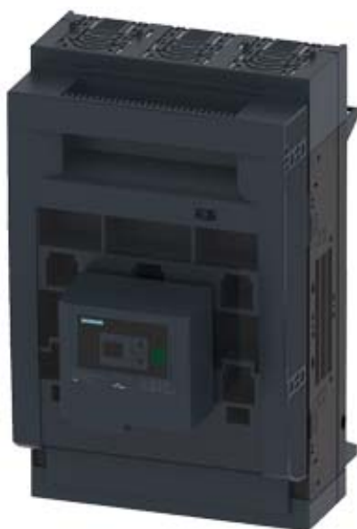
FUSE-SWITCH-DISCONNECTOR 3-POLE, NH1, 250A 60MM BUSBAR SYSTEM COVERS FOR RITTAL BOX TERMINAL FUSE MONITORING ELECTRONIC, EFM 20
