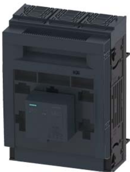
FUSE-SWITCH-DISCONNECTOR 3-POLE, NH2, 400A 60MM BUSBAR SYSTEM COVER LEVEL 32/70 MM FLAT CONNECTOR FUSE MONITORING ELECTRONIC, EFM 10
