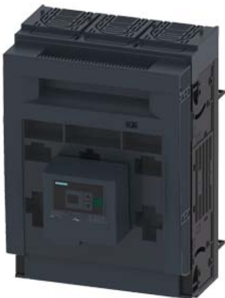
FUSE-SWITCH-DISCONNECTOR 3-POLE, NH2, 400A 60MM BUSBAR SYSTEM COVER LEVEL 32/70 MM FLAT CONNECTOR FUSE MONITORING ELECTRONIC, EFM 20
