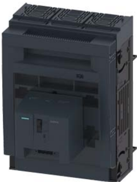
FUSE-SWITCH-DISCONNECTOR 3-POLE, NH2, 400A 60MM BUSBAR SYSTEM COVER LEVEL 32/70 MM BOX TERMINAL FUSE MONITORING ELECTROMECHANICAL
