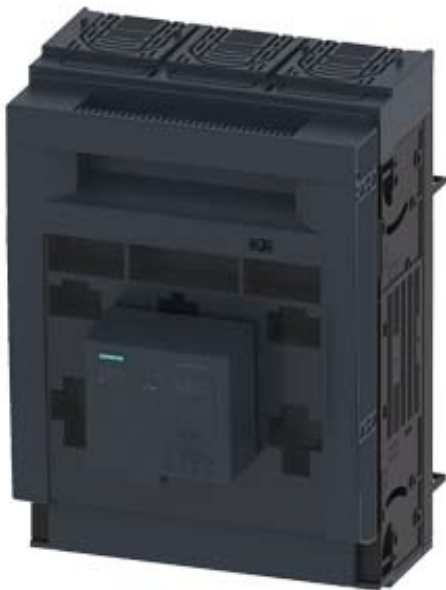
FUSE-SWITCH-DISCONNECTOR 3-POLE, NH2, 400A 60MM BUSBAR SYSTEM COVER LEVEL 32/70 MM BOX TERMINAL FUSE MONITORING ELECTRONIC, EFM 10
