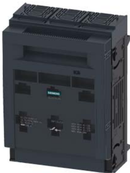
FUSE-SWITCH-DISCONNECTOR 3-POLE, NH2, 400A 60MM BUSBAR SYSTEM COVERS FOR RITTAL BOX TERMINAL
