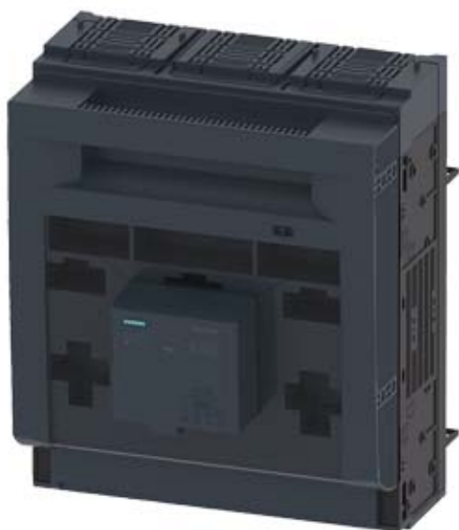
FUSE-SWITCH-DISCONNECTOR 3-POLE, NH3, 630A 60MM BUSBAR SYSTEM COVER LEVEL 32/70 MM FLAT CONNECTOR FUSE MONITORING ELECTRONIC, EFM 10
