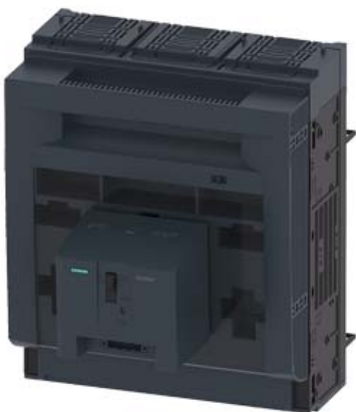
FUSE-SWITCH-DISCONNECTOR 3-POLE, NH3, 630A 60MM BUSBAR SYSTEM COVER LEVEL 32/70 MM BOX TERMINAL FUSE MONITORING ELECTROMECHANICAL
