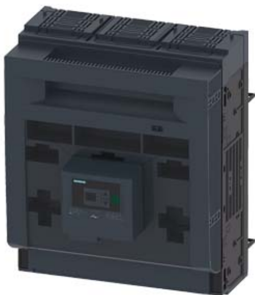
FUSE-SWITCH-DISCONNECTOR 3-POLE, NH3, 630A 60MM BUSBAR SYSTEM COVER LEVEL 32/70 MM BOX TERMINAL FUSE MONITORING ELECTRONIC, EFM 20
