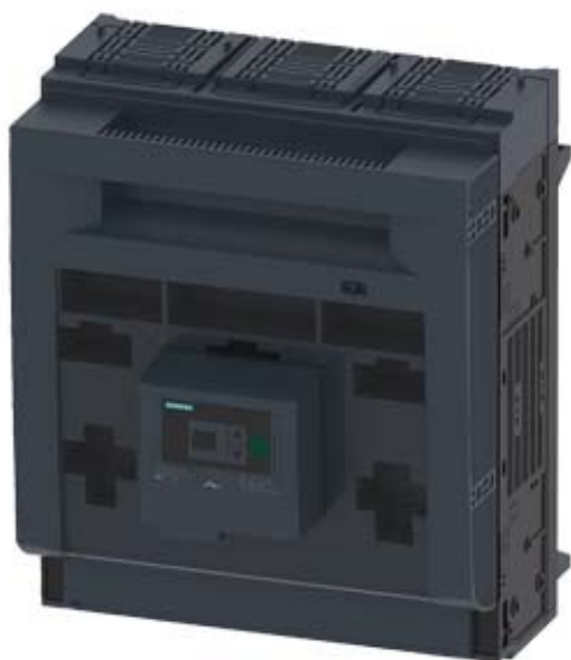
FUSE-SWITCH-DISCONNECTOR 3-POLE, NH3, 630A 60MM BUSBAR SYSTEM COVERS FOR RITTAL FLAT CONNECTOR FUSE MONITORING ELECTRONIC, EFM 20
