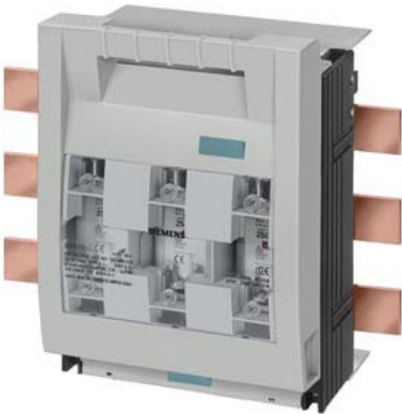
FUSE-SWITCH-DISCONNECTOR I = 100/160A, U = 500/400V FOR 40MM BUSBAR RAISED ADAPTER BOX TERMINAL AT TOP FUSE SIZE NH00 HANDLE
