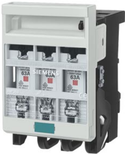
FUSE-SWITCH-DISCONNECTOR I = 100/160A, U = 500/400V FOR 40MM BUSBAR FLAT ADAPTER BOX TERMINAL AT BOTTOM FUSE SIZE NH000 HANDLE
