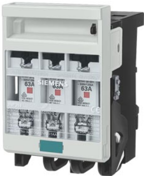
FUSE-SWITCH-DISCONNECTOR I = 100/160A, U = 500/400V FOR 40MM BUSBAR FLAT ADAPTER BOX TERMINAL AT TOP FUSE SIZE NH000 HANDLE
