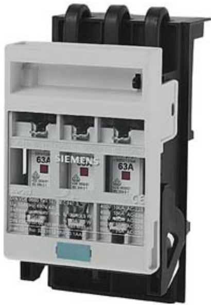
FUSE-SWITCH-DISCONNECTOR I = 100/160A, U = 500/400V FOR 60MM BUSBAR ADAPTOR FLAT, BOX TERMINAL AT BOTTOM FUSE SIZE NH000
