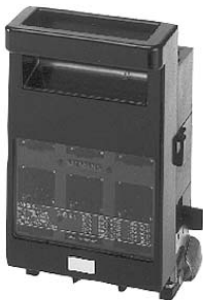
FUSE-SWITCH-DISCONNECTOR I=160A, U=690V, 3-POLE WITH CLAMP CONNECTION FUSE SIZE NH00
