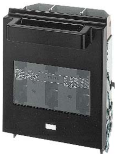
FUSE-SWITCH-DISCONNECTOR I=250A, U=690V, FUSE SIZE NH0 AND NH1 WITH CLAMP CONNECTION
