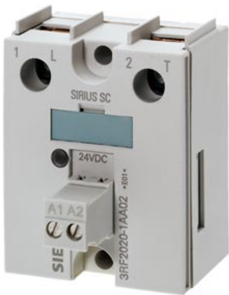
SEMICONDUCTOR RELAY 3RF2, 1-PH. WIDTH 45 MM, 20 A 24-230 V / 24 V DC SCREW TERMINAL
