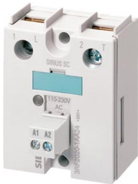
SEMICOND. RELAY 3RF2, 1-PHASE WIDTH 45 MM, 90 A 24-230 V / 110-230 V AC SCREW TERMINAL
