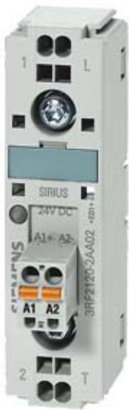
SEMICOND. RELAY 3RF2, 1-PHASE WIDTH 22.5 MM, 20 A 24-230 V / 110-230 V AC SPRING-LOADED TERMINAL
