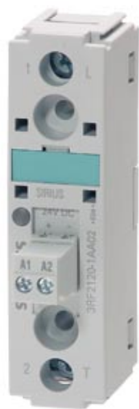
SEMICOND. RELAY 3RF2, 1-PHASE WIDTH 22.5 MM, 50 A 24-230 V / 110-230 V AC SCREW TERMINAL
