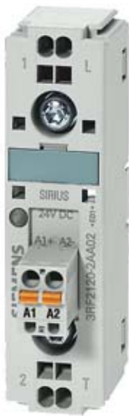
SEMICONDUCTOR RELAY 3RF2, 1-PH. WIDTH 22.5MM, 90 A 48-460 V / 110-230 V AC SPRING-LOADED TERMINAL
