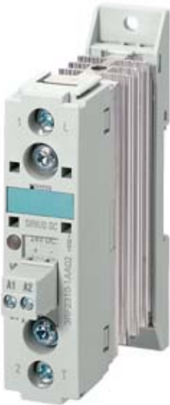
SEMICOND. CONTACTOR 3RF2, 1-PH. AC51 10.5 A 40 DEG. C 24-230V / 24V AC/DC SCREW CONNECTION
