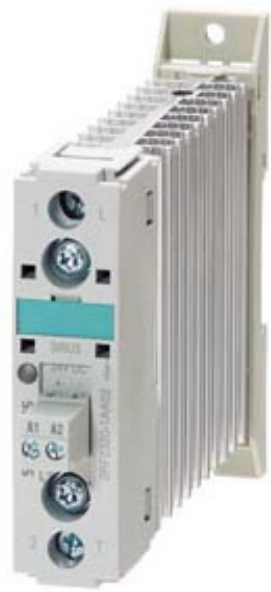
SEMI-COND. CONTACTOR 3RF2,1-PH. AC 51 20 A 40 DEGREES C 24-230 V / 24 V DC SCREW TERMINAL
