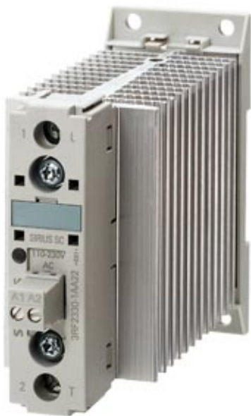
SOLID-STATE CONTACTOR 3RF2,1-PH AC51 30A 40 DEGR. C 48-600V / 110-230VAC SCREW CONNECTION BLOCKING VOLTAGE 1200V
