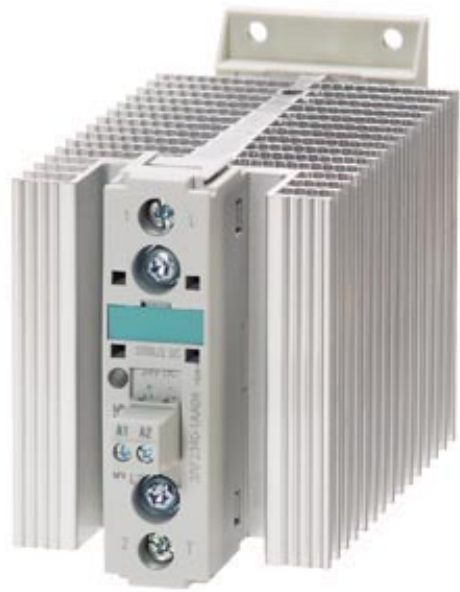
SOLID-STATE CONTACTOR 3RF2,1-PH AC51 40A 40C 48-600V / 4-30V DC SCREW-TYPE TERMINAL BLOCKING VOLTAGE 1200V
