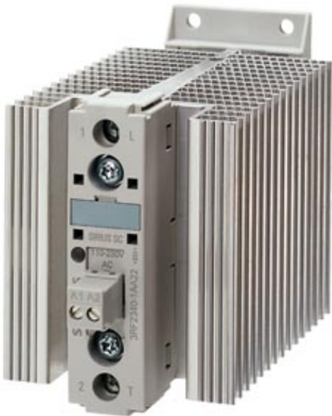
SEMI-COND. CONTACTOR 3RF2,1-PH. AC 51 50 A 40 DEGREES C 48-460 V / 24 V DC SCREW TERMINAL
