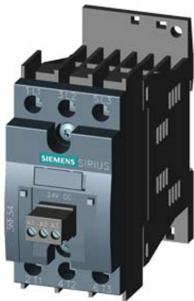
SOLID-STATE CONTACTOR 3-PH 3RF3 AC53 3.8A 40 DEGREES C 48-480V / 24V DC REVERSE SWITCHING INSTANTANEOUS SCREW TERMINALS
