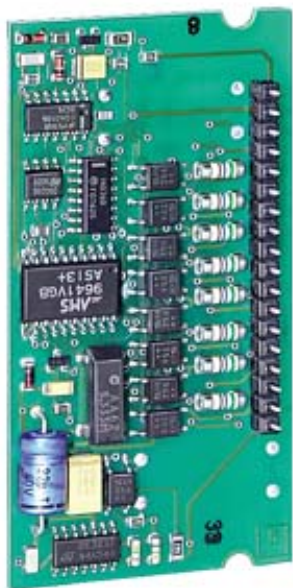
AS-INTERFACE MODULE 4I/4O, PNP FOR PRINTED CIRCUIT BOARD WITH SOLDER PINS
