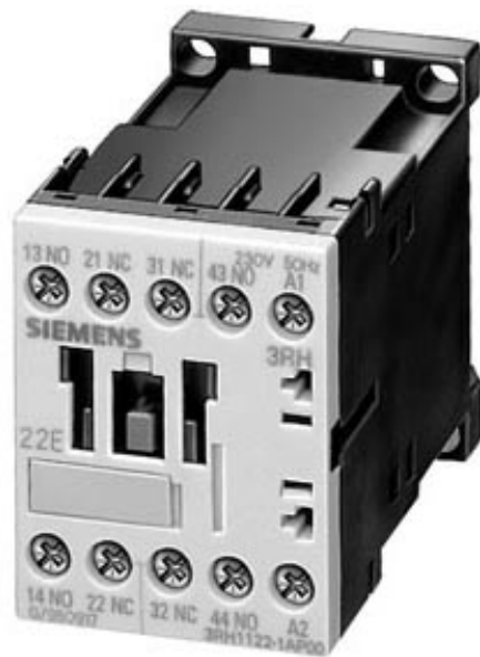
CONTACTOR RELAY, 2 NO + 2 NC, AC 400 V 50HZ/400...440V 60HZ, SCREW-TYPE CONNECT., MOD. S00
