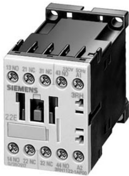
CONTACTOR RELAY, 3NO+1NC, 400 V AC, 50 HZ/ 440 V AC, 60HZ SCREW CONNECTION, SIZE S00
