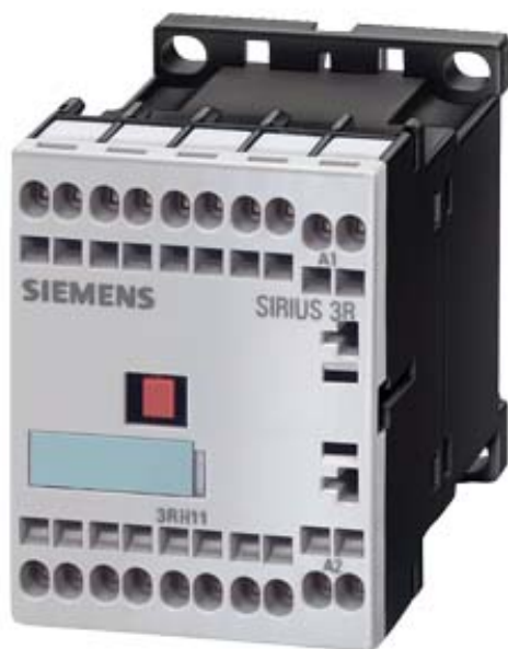
CONTACTOR RELAY, 3NO+1NC, DC 48 V, CAGE-CLAMP CONNECTION, SIZE S00
