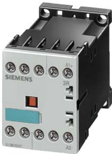
COUPLING RELAY F. AUXILIARY CIRCUITS, 4NO, 24V DC, SIZE S00, 0.85...1.85XUS, 1.4W, SCREW CONNECTION, DIODE BUILT-IN
