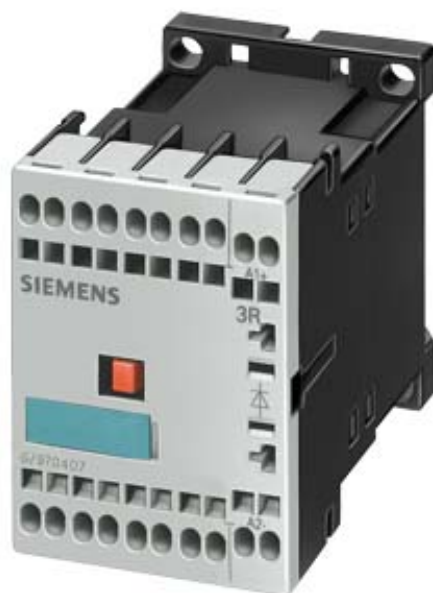
COUPLING RELAY, 4NO, DC 24 V, 0.7...1.25*US, CAGE CLAMP CONNECTION, SIZE S00
