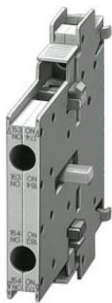
AUX. SWITCH BLOCK, 1 NO+1 NC, DIN EN50012, LATERALLY, 10 MM SCREW CONNECTION, SIZE S3...S12 FOR MOTOR CONTACTORS, 2-POLE
