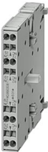
AUX. SWITCH BLOCK, 1NO + 1NC, DIN EN 50012, LATERAL, 10MM, CAGE CLAMP, FOR MOTOR CONTACTORS, SIZE S0...S12
