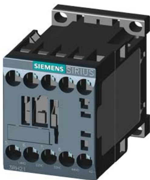
CONTACTOR RELAY, 2NO+2NC, DC 12V, SIZE S00, SCREW TERMINAL
