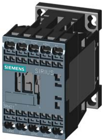
CONTACTOR RELAY, 2NO+2NC, AC 220V 50HZ, 240V 60HZ, SZ S00, SPRING-LOADED TERMINAL
