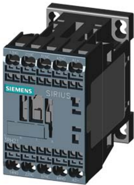
CONTACTOR RELAY, 2NO+2NC, DC 24V, SZ S00, SPRING-LOADED TERMINAL
