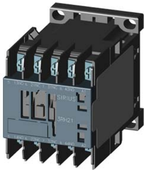
CONTACTOR RELAY, 2NO+2NC, AC 24V, 50/60 HZ, SZ. S00, RING CABLE LUG CONNECTION
