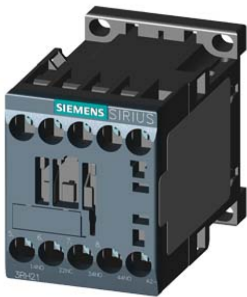
COUPLING CONTACTOR RELAY, 3NO+1NC, DC 24V, 0.7...1.25*US, W/ INTEGRATED DIODE, SIZE S00, SCREW TERMINAL
