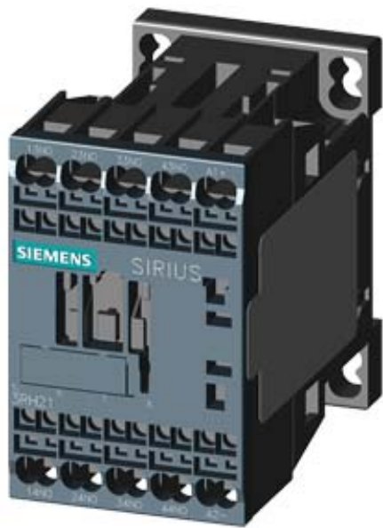
CONTACTOR RELAY, 4NO, DC 60V, SZ S00, SPRING-LOADED TERMINAL
