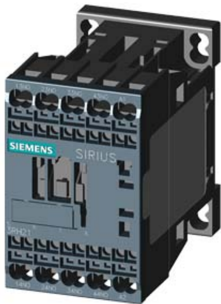
CONTACTOR RELAY, 4NO, AC 110V, 50/60 HZ, W/ FULL-WAVE RECTIFIER, SZ S00, SPRING-LOADED TERMINAL
