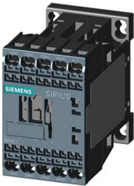
COUPLING CONTACTOR RELAY, 4NO, DC 24V, 0.85...1.85*US, W/ INTEGRATED DIODE, SZ S00, SPRING-LOADED TERMINAL
