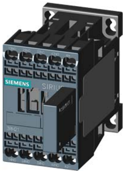
COUPLING CONTACTOR RELAY, 4NO, DC 24V, 0.85...1.85*US, W/ PLUGGED-ON VARISTOR, SZ S00, SPRING-LOADED TERMINAL
