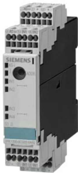
AS-INTERFACE MODULE SLIMLINE S22.5, DIGITAL, 4I, 2-WIRE,IP20 4 X 1 INPUT, 2-WIRE, PNP CAGE-CLAMP, MODULE WIDTH 22.5 MM
