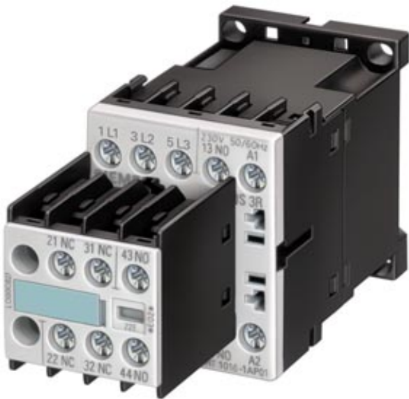
CONTACTOR, AC-3 4 KW/400 V, 1 NO, AC 24 V, 50/60 HZ, 3-POLE, SIZE S00, SCREW CONNECTION
