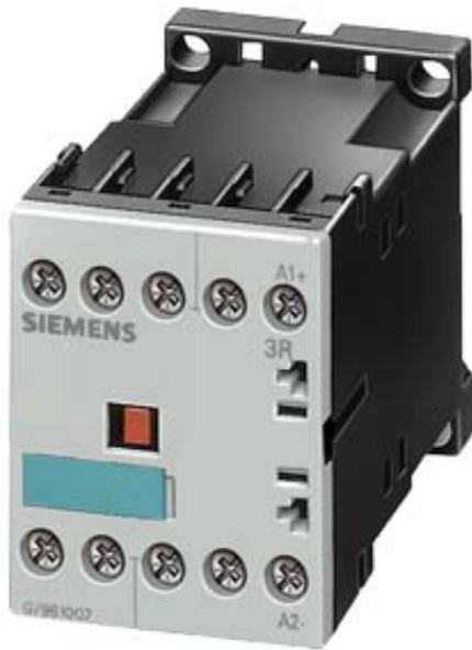
COUPLING RELAY, AC-3 4 KW/400 V, 1 NC, DC 24 V, 0.7...1.25*US, W.DIODE 3-POLE, SIZE S00, SCREW CONNECTION
